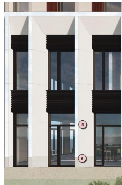
Image 76 (above): Ground and first floor bays of Building A/B, highlighting at (5) the white metal piers and at (6) the textured metal footers.
