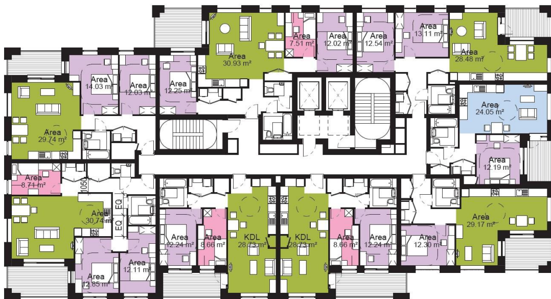
Image 57 (above): Layout of Levels 02-07 of Building D, showing the range of home sizes that would be provided and their layouts.
