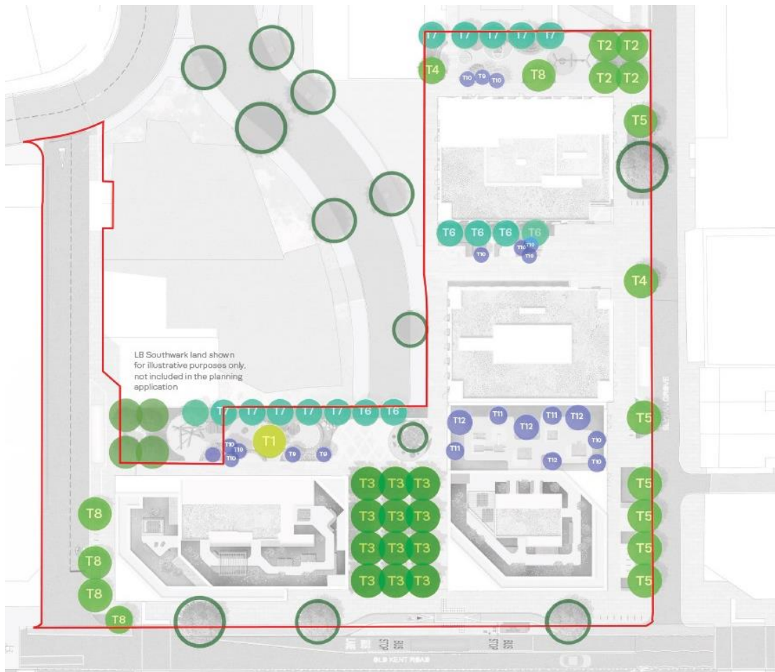
Image 103 (above): Site layout showing the arrangement and variety of the 68 trees proposed. The deep and mid-greens indicate large/medium sized trees, whereas blue and mint green indicate smaller naturalistic or feature trees.
